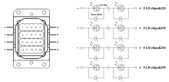
Fig.3 20LD chips Drive Circuit
