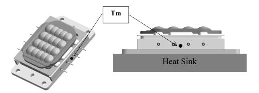
Fig.1 Schematic diagram of measurement system
