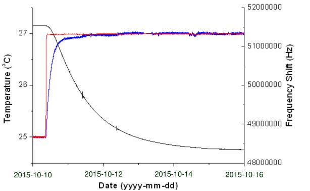
Red: temperature of the copper case Blue: temperature outside of the vacuum chamber Black: Beat frequency
